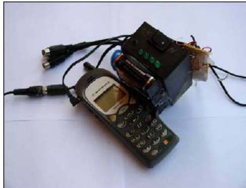
A wireless detonation system based on a cellular telephone, for a chain detonation of up to four IEDs
